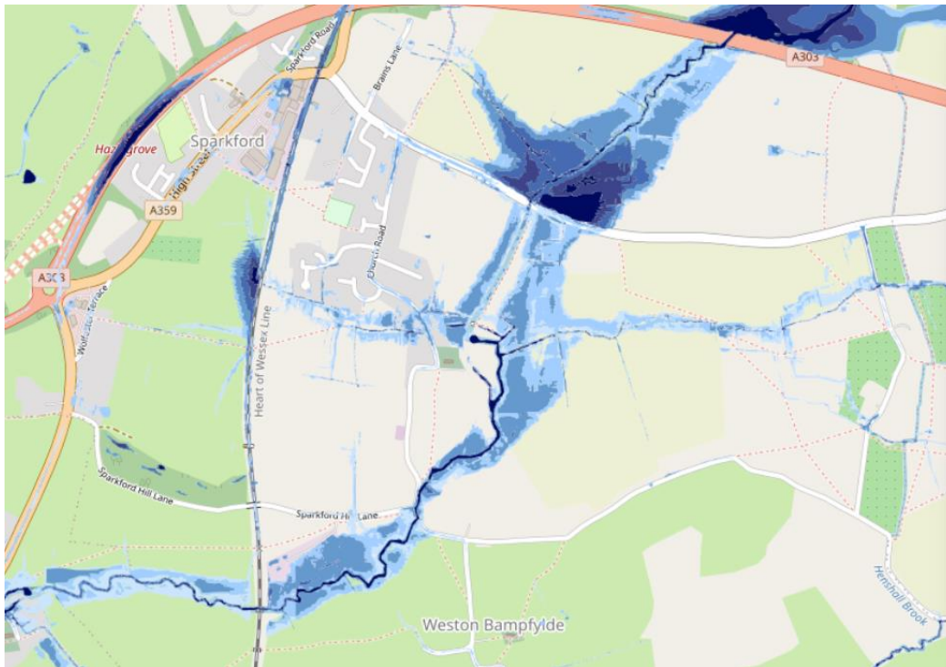
Figure 18 Defra OGC map of Sparkford & Weston Bampfylde - Risk of Flooding from Surface Water Depth: 0.1% annual chance
