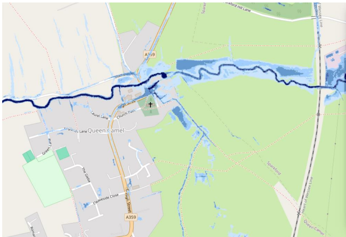
Figure 19 Defra OGC map of Queen Camel - Risk of Flooding from Surface Water Depth: 0.1% annual chance
